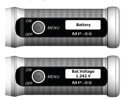
If the battery voltage drops below 1.0V, the device switches off automatically.
