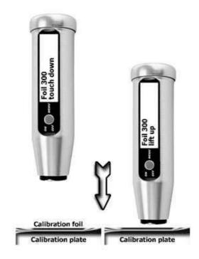
If possible, the **calibration foil with the higher value (approx. 300 \mum)** should always be used for calibration in order to maintain the specified accuracy of the instrument over the **entire measuring range**.
