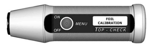
Place the approx. 300  $\mu$ m calibration foil on the bare FE / NFE calibration base plate. In the raised state activate **FOIL CALIBRATION**, then apply the device with the measuring probe to the measuring foil and wait until the foil value is displayed and confirmed by a long sound on FE or two short sounds on NFE.
