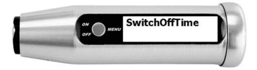
Selection of the automatic switch-off time of the device (5 minutes / 10 minutes /. 30 minutes / off = the device is always switched on). Off should only be selected in special cases, as this can greatly increase the power consumption.
