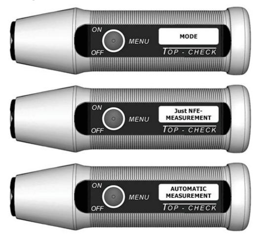
**AUTOMATIC MEASUREMENT** is switched on as standard. The measuring probe recognizes the base material (FE or NFE) and automatically switches to the correct measuring mode (magnetic-inductive on FE or eddy current method on NFE).
