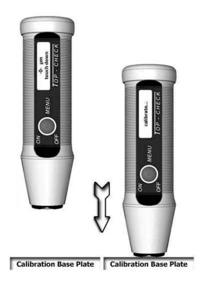
If you have to measure **on materials other than flat steel or aluminum**, please perform the calibration on an uncoated original part instead of on the calibration base plate. This applies in particular to curvatures, round material or special alloys.
