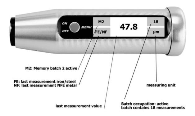
The measurement display shows the last measured value and its measuring unit at a glance. At the bottom left, it indicates whether the measurement was taken on iron/steel (FE = ferromagnetic, FE metal) or on non-ferromagnetic metal (NF = NFE metal).
