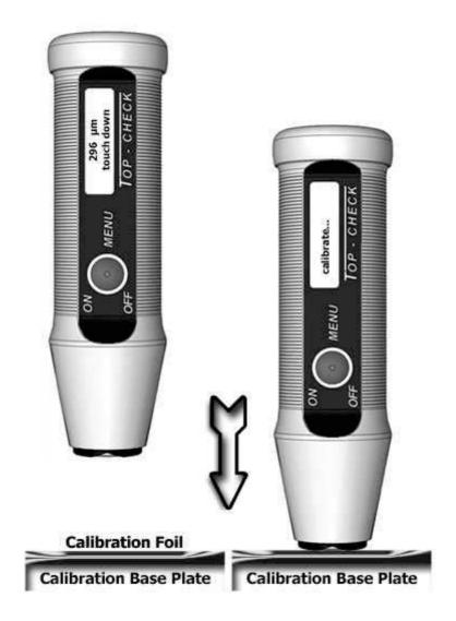
The measuring foil with the higher value (approx. 300  $\mu$ m) should always be used for an accurate calibration of the whole measuring range. The calibration for FE measurements is carried out on the blue FE base plate, the calibration for NFE measurements on the red NFE base plate.
