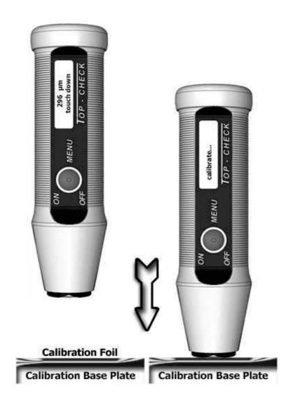
The measuring foil with the higher value (approx. 300  $\mu$ m) should always be used for an accurate calibration of the whole measuring range.
