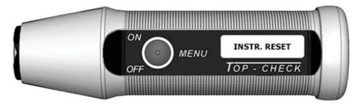
If the device can no longer be calibrated properly or if other malfunctions occur the works calibration can be restored here by means of an instrument reset. When doing this the device switches off automatically.
