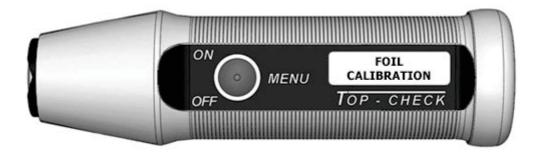
Place the approx. 300  $\mu$ m calibration foil on the bare FE calibration base plate. In the raised state activate **FOIL CALIBRATION**, then apply the device with the measuring probe to the measuring foil and wait until the foil value is displayed and confirmed by a long sound.
