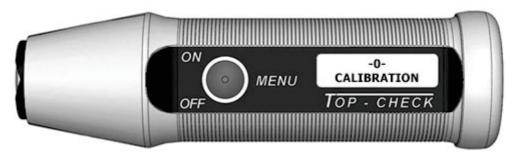
In the raised state activate **-0- CALIBRATION**, then apply the device with the measuring probe to the bare FE calibration base plate and wait until  $0.0~\mu m$  is displayed and confirmed by a long sound.
