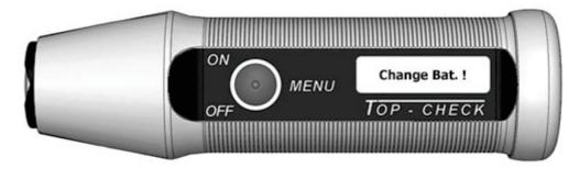
The battery must be replaced as soon as the warning **Change Bat.** Appears.
