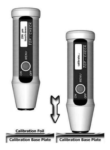
The measuring foil with the higher value (approx. 300  $\mu$ m) should be always used for an accurate calibration of the whole measuring range. The calibration for FE measurements is carried out on the blue FE base plate, the calibration for NFE measurements on the red NFE base plate.
