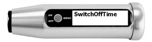
Selection of the automatic switch-off time of the device (5 minutes / 10 minutes /. 30 minutes / off = the device is always switched on). Off should only be selected in special cases, as this can greatly increase the power consumption.
