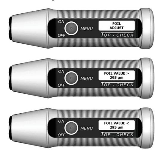
A short press of the button changes the foil value in 1  $\mu$ m steps; after releasing the button for at least 1 second, the < sign switches to > and back in order to increase or decrease the foil value.
