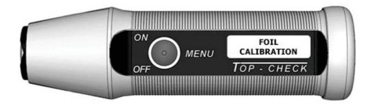
Place the approx. 300  $\mu$ m calibration foil on the bare FE / NFE calibration base plate. In the raised state activate **FOIL CALIBRATION**, then apply the device with the measuring probe to the measuring foil and wait until the foil value is displayed and confirmed by a long sound on FE or two short sounds on NFE.
