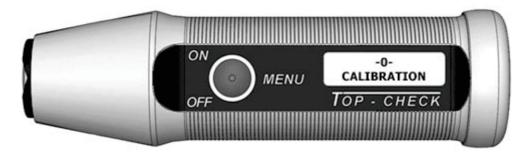
In the raised state activate **-0- CALIBRATION**, then apply the device with the measuring probe to the bare FE / NFE calibration base plate and wait until 0.0  $\mu$ m is displayed and confirmed by a long sound on FE or two short sounds on NFE.
