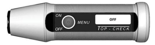
The device is manually switched off by pressing and holding the button (long sound). If the button is kept pressed for more than 3 seconds after switching off, then the program version is displayed before the device switches off.
