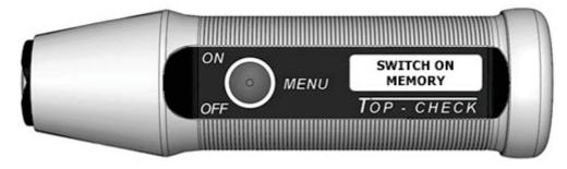
Switches the memory / data logger on or off.
