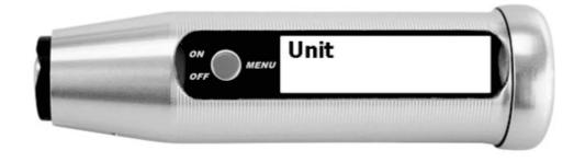
Change of the measuring unit between  $\mu m$  and mil (1 mil = 25.4  $\mu m$ ). The active measuring unit is displayed with an asterisk (\*) behind the entry.
