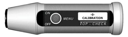
In the raised state activate **-0- CALIBRATION**, then apply the device with the measuring probe to the bare FE / NFE calibration base plate and wait until 0.0  $\mu$ m is displayed and confirmed by a long sound on FE or two short sounds on NFE.
