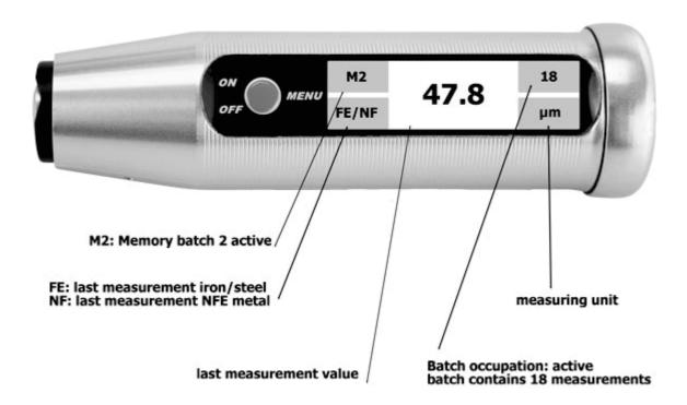
The measurement display shows the last measured value and its measuring unit at a glance. At the bottom left, it indicates whether the measurement was taken on iron/steel (FE = ferromagnetic, FE metal) or on non-ferromagnetic metal (NF = NFE metal).
