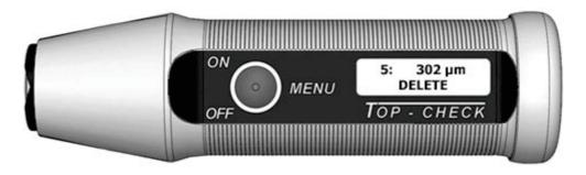
You can confirm the deletion of the measured value by pressing and holding the button, or return to the display of the individual measured values without deleting it by a short press of the button.
