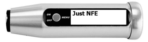
**Just NFE** is a measurement mode for non-ferrous metals such as aluminum, brass and as a special feature also for stainless steel. Here, only the eddy current method is used for measurement.
