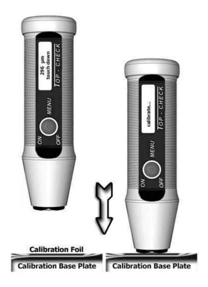
The measuring foil with the higher value (approx. 300  $\mu$ m) should be always used for an accurate calibration of the whole measuring range. The calibration for FE measurements is carried out on the blue FE base plate.
