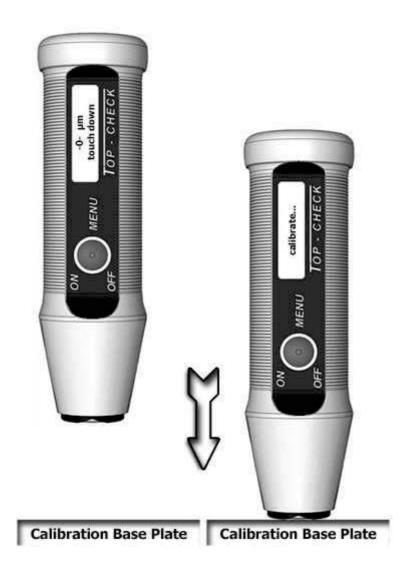
If you have to measure **on materials other than flat steel**, please perform the calibration on an uncoated original part instead of on the calibration base plate. This applies in particular to curvatures, round material or special alloys.
