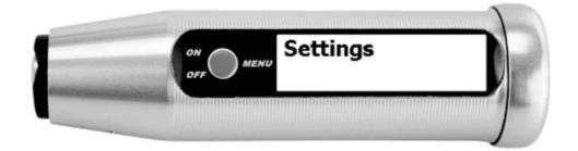
In the settings menu, you can set the language, measuring unit, measuring type, switch-off time, volume and contrast for your device. These settings are retained even after the device is switched off. These settings are deleted during a factory device reset.
