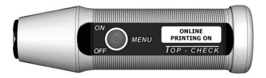
With a long press on the red button, you can change the printing mode to either **printing on**, or **printing off**.
