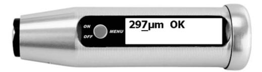
Second step: the bar is under a number. Now press and hold, the number starts to flash. Now press briefly until the desired value is reached. Then press and hold again to accept the new value. The bar moves under the next field.
