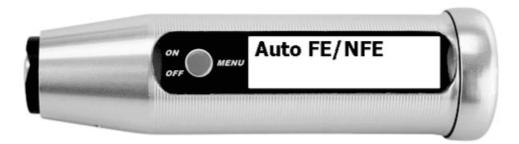
With **Auto FE/NFE** the probe recognizes the base material (FE like ferro-magnetic, iron/steel or NFE non-ferromagnetic like aluminum/brass) and automatically switches to the correct measuring method (magnetic inductive / eddy current). For measurements on <u>stainless steel</u> please read the section **Just NFE**.
