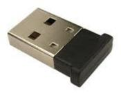
For TOP-CHECK FE-B and TOP-CHECK FN-B a Bluetooth dongle is included as shown.
